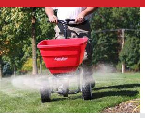
The EV-N-SPRED<sup>®</sup> Dual Port PRO Adjustable Shut-Off System is included on all Professional models and allows the operator to balance the spread pattern evenly across the full 180° spread width, regardless of the weight or size of granular material. By closing either the right and/or left side throwing ports, you can balance the spread pattern to exacting precision without compromising spread width to application rate.
