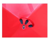
**CONFIRM THE CALIBRATION:**Lever at #30 and the drop holes fully open
